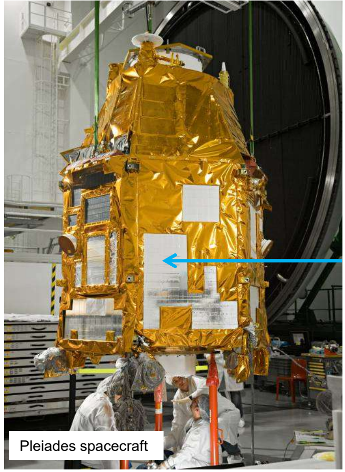
Radiators with SSM
