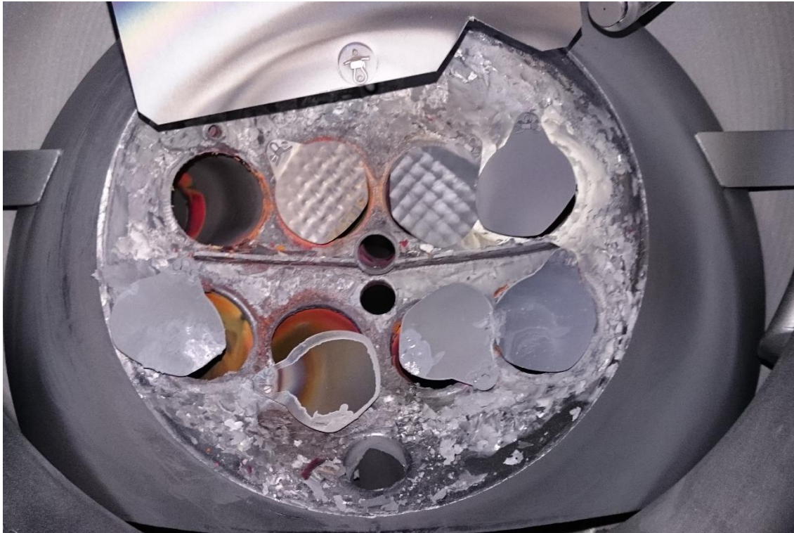
Cell cryopanel with material residues
