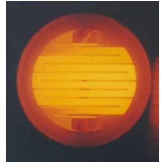
Hot graphite filament : up to 2300°C
