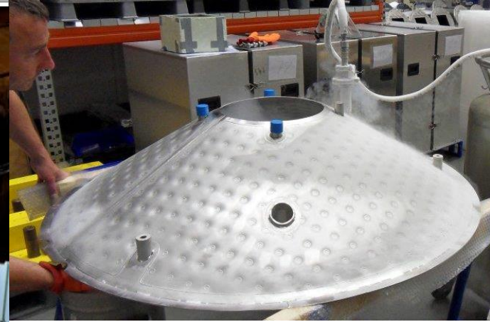
Hydro-formed thermal shield undergoing 80K thermal cycle.
