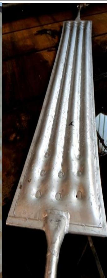
4.5 K Cryopanel after 130 bar burst test
