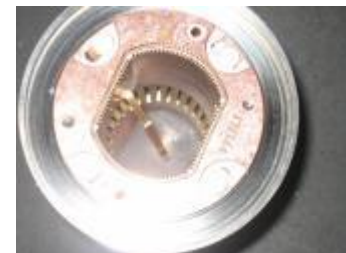
A buckled PIM
